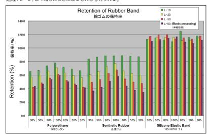
This phenomenon is due to the fact that the stretch force retention at 100% elongation after 50-cycle treatment is 61.8% for polyurethane and 68.0% for synthetic rubber, where the force is reduced in both cases, however, 114% for silicone, where the force has increased.
