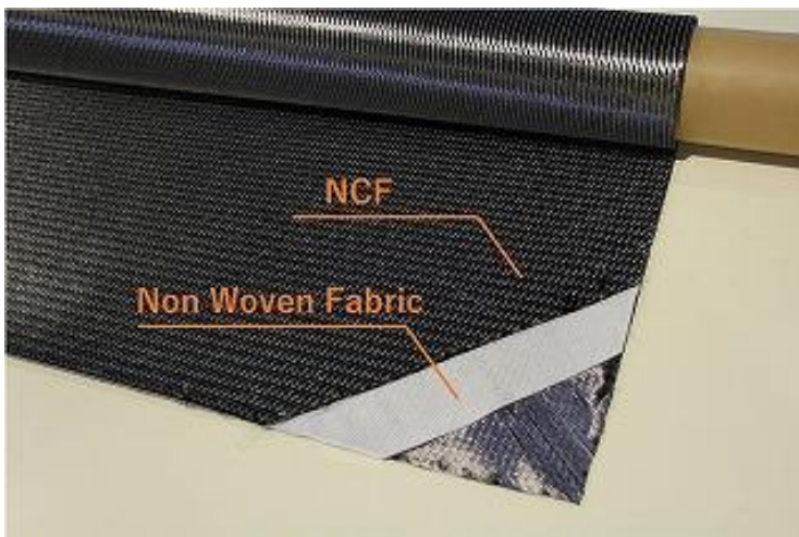
Fig. 1 A fabric comprising a thermoplastic layer embedded between noncrimp fabric (NCF) layers.
