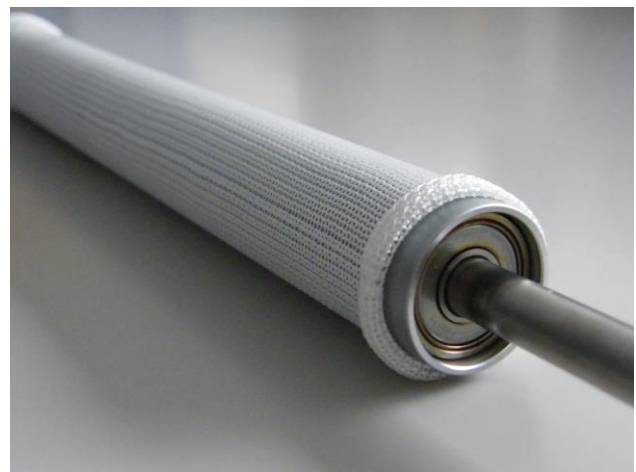
Fig. 9 Covered roller application of our tailored cylindrical fabric.
