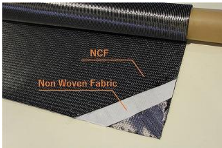
Fig. 1 The fabric that a thermoplastic layer is inserted to NCF layers.
